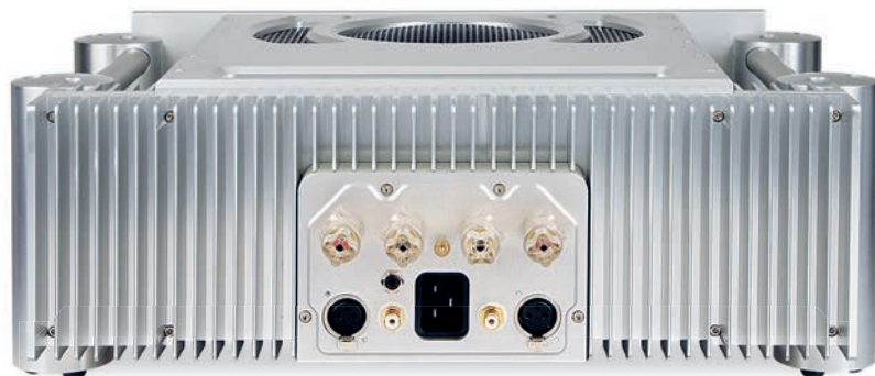
ABOVE: Unmarked, but explained in the manual, the right-hand RCA and XLR input(s) provide a non-inverting output, the left-hand RCA/XLR inputs an inverting output. Only one input may be used but the 4mm speaker outlets are paralleled for bi-wiring
